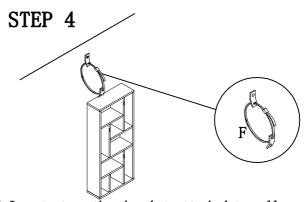
1. Insert strap thru bracket attached to wall. then thru bracket on item, and into head of strap. 2. pull lightly til strap stops.
