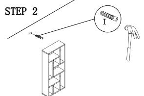
1. Use a light hammer to tap anchor into hole. 2. Anchor should fit snugly. If hole is too small, drill again to increase hole size . Do not force anchor into wall.
