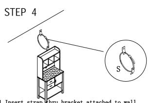
1. Insert strap thru bracket attached to wall.
