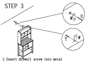
bracket and into drywall anchor.
