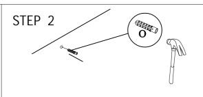
1.Use a light hammer to tap anchor into hole.
