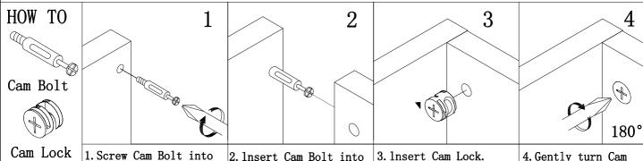
1. Screw Cam Bolt into panel.
